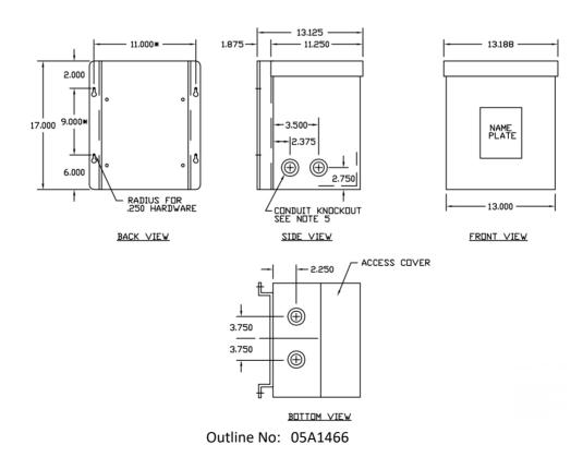
Meets 10 CFR 431(2016) Efficiency Dry Type Transformer General Purpose
